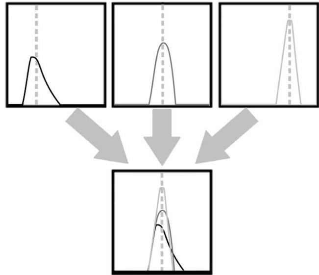
Fig. 2. Offsetting of the V-Group histogram, where the mean maximum reflectance value shown as the dotted line is centralized for each case
