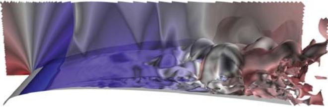
Fig. 3. Instantaneous situation of the CFD result in the transonic buffet on the wing upper region. We illustrate the wing upper surface, iso-surface of turbulent viscosity with  $C_p$  distribution, and the surface at  $y = 0.40$  with  $C_p$  distribution.
