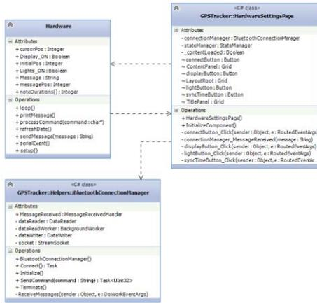
Figure 1: Class diagram of notification hardware
