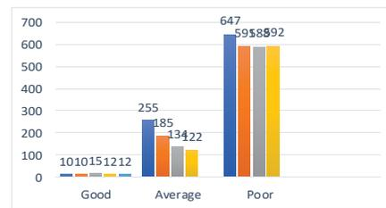
Figure 2: Location Accuracy vs. Signal Strength
