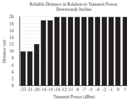
Figure 8. Minimal obstructions on an downwards incline. This graph maps to experiment II.
