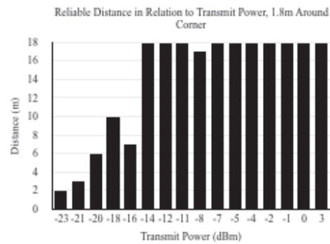
Figure 11. Minimal obstructions around a corner, 184cm along the wall. This graph maps to experiment V.
