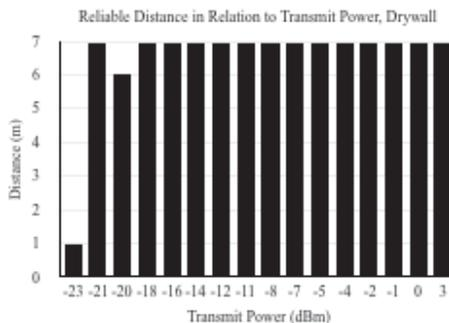
Figure 10. Minimal obstructions through 166cm drywall and space. This graph maps to experiment IV.
