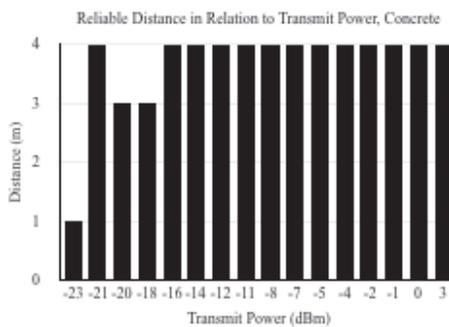
Figure 9. Minimal obstructions through a 182cm concrete wall. This graph maps to experiment III.
