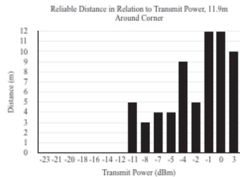
Figure 12. Minimal obstructions around a corner, 1191cm along the wall. This graph maps to experiment VI.
