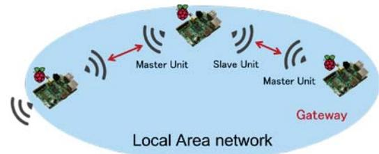
Fig.10 Network configuration of the proposed system
