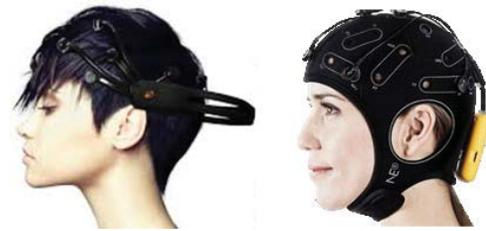
Fig 2 Head set type (EMOTIVE) and head cap type (ENOBIO) electroencephalographs
