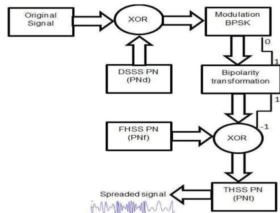
Fig. 5. Hybrid Spread Spectrum Approach.
