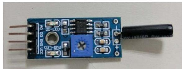
Figure 3. Vibration sensor of the embedded device.
