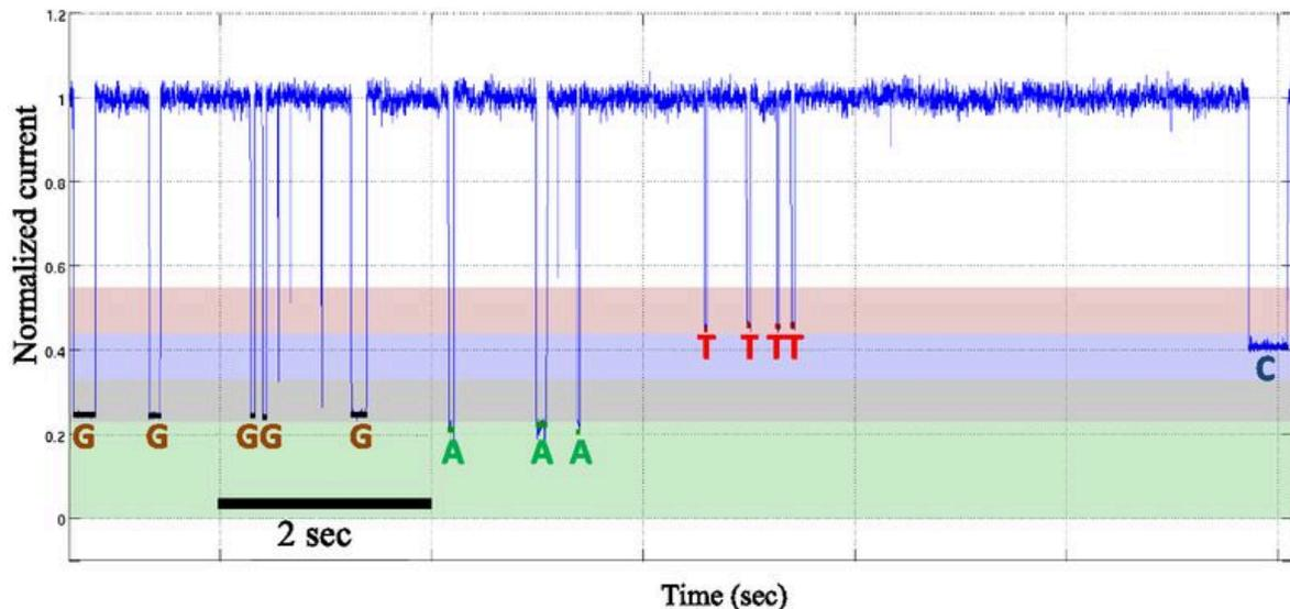
This image shows single-molecule nanopore DNA sequencing by synthesis data from a template with homopolymer sequences<sup>4</sup>.
