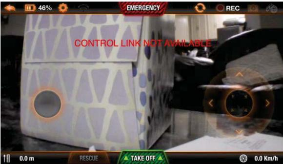
Fig. 5. Communication link after dos attack
