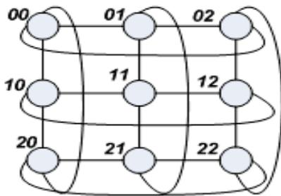
**Figure 1:** 2-D Torus,  $Q_2^3$ , that contains an  $3^2$  nodes, three in each row or column
