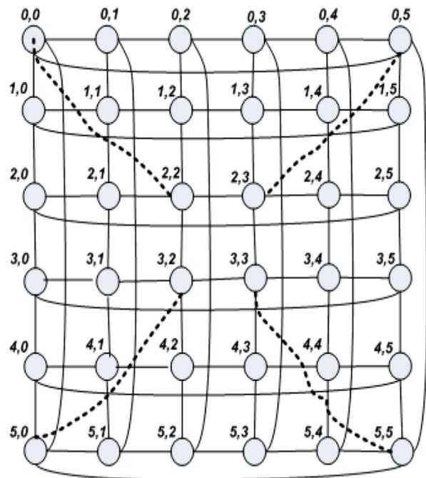
**Figure 2:**  $C^2$ Torus;  $C2_2^n$ ; that contains an  $n^2$  nodes with four center nodes
