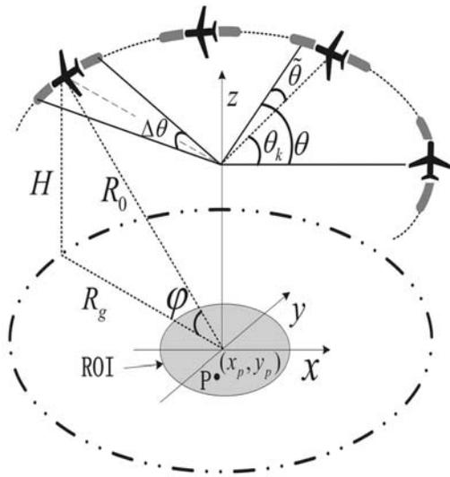
Fig. 1 ViSAR geometry [1].
