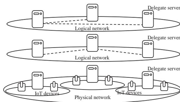
Fig. 1: Architecture of multi-layered IoT service platform
