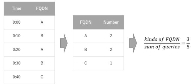
Fig. 5: Calculation example of diff rate
