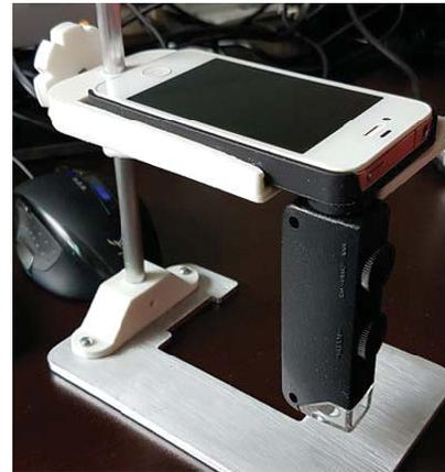
Fig. 5: Data acquisition system using smart phone.
