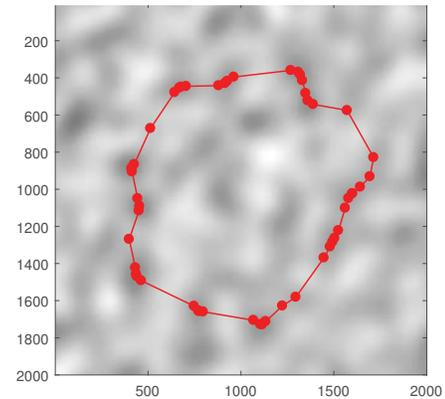
Fig. 1. Examples of a path generated by the original ENA on a random map. Darker colors represent regions with higher resource abundance. Nodes are strongly drawn to peaks on the map instead of spreading evenly as intermediate points. Thus the separation constraints are broken.
