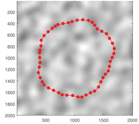
Fig. 2. Examples of a path generated by our algorithm with barrier functions, on the same random map as in Fig.1. With the help of barrier functions, the constraints can be maintained and the nodes are more evenly distributed.
